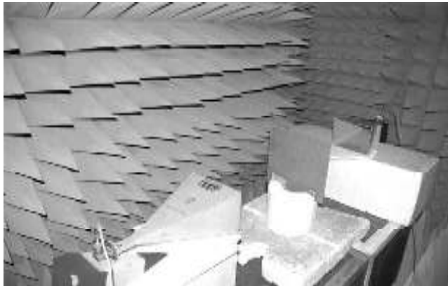
Fig. 8. FSS radome testing in the anechoic chamber.
