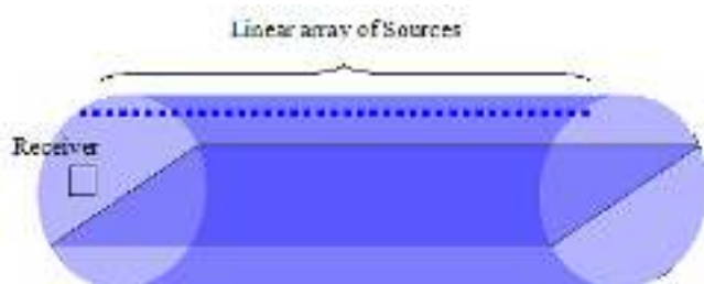
Fig 1: Schematic of LCX antenna modeled by linear array of sources inside the elliptic cylindrical aircraft cabin.
